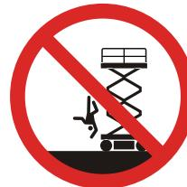
Prevent falling from the platform. Always keep a firm footing on the platform floor when working thereon. Do not climb on the toe-board, mid-rail, or top-rail. Do not use planks, ladders, or any other devices on the platform for achieving additional height or reach.
