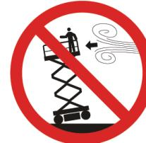
**DO NOT** raise the platform or operate elevated in windy or gusty conditions that exceed the limits specified in [Section 7.5](#).
