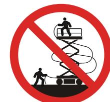
**DO NOT** allow the entanglement of ropes, cables or hoses with the MEWP, adjacent structures or objects.
