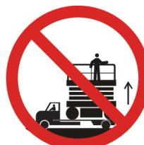
**DO NOT** elevate the platform when the MEWP is on a truck, forklift, or other device or vehicle.
