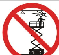
**DO NOT** collide or crush. Be aware of obstructions, personnel, or other possible hazards around the MEWP when elevating, lowering, or driving. Keep all body parts inside the platform when elevating or driving. Be aware of blind spots when operating the MEWP.
