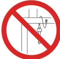
**DO NOT** use the MEWP without guardrails, lock-pins, and the entry gate(s) in place.
