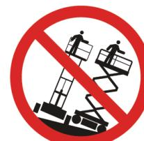
**DO NOT** elevate or drive elevated on a slope. Elevated driving must be done on a firm, level surface.
