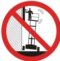
**DO NOT** exceed the maximum side force on the platform capacity label when elevated (refer to [Section 7.5](#)).
