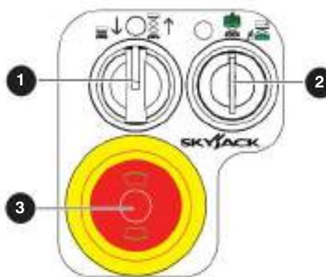
**1 Lower/neutral/raise:** This switch controls the function to lower or raise the platform.
