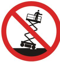
**DO NOT** drive elevated near depressions or holes of any type, loading docks, debris, drop-offs or surfaces that may affect the stability of the MEWP.
