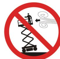
**DO NOT** increase the surface area of the platform or carry large surface area items when exposed to wind. Increasing the area exposed to the wind will decrease the MEWP stability.
