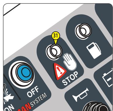
If flashes when a fault is detected:
