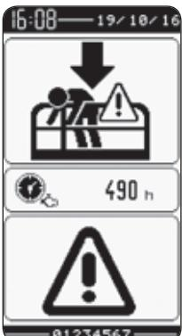
This ALARM PAGE is displayed when the platform is powered up without starting the engine in the next 10 seconds.
