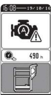
This ALARM PAGE is displayed when the engine is stopped by the ENGINE AUTOMATIC STOP SYSTEM "STOP AND GO" and when the engine must be restarted immediately,
