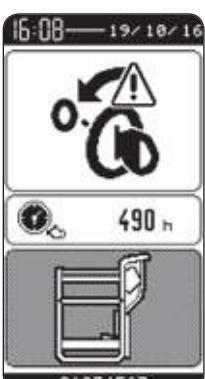
This ALARM PAGE is displayed when the engine is stopped by the ENGINE AUTOMATIC STOP SYSTEM "STOP AND GO",
