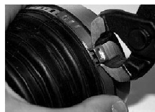
Fit clip over application. Engage interlocking hooks in tightest available position. Firmly crimp the ear with pincers.
