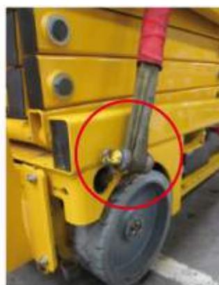
The slings must be positioned from inside of the railings as shown below.
