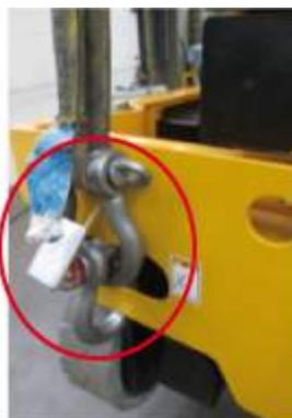
Hook 1 - 2 T shackle with a sling 3 m (9 ft 10 in) 3 T to each hole at the rear of the machine.
