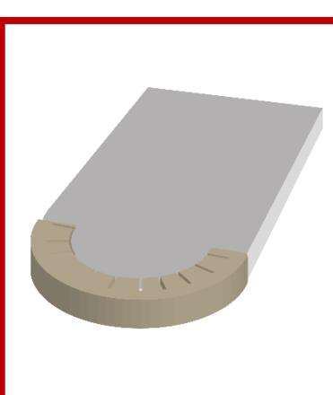
Notched on one leg to protect the edge of a curved object
